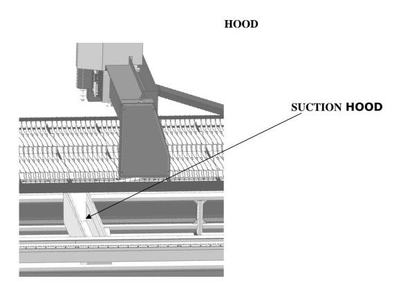
The suction hood is a type of container which travels with the gantry, concentrating the suction below the work area, thereby reducing operating and investment costs, and significantly reducing the power required for the suction unit.
