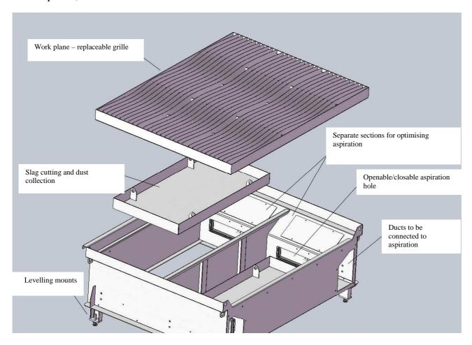
To achieve correct aspiration it is necessary to have a depression output equivalent to that given by the fan.
