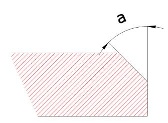
When the inclined portion, **a** acts on the entire thickness, the cut is made in a single pass, otherwise it is necessary two; one for each cutting angle.
